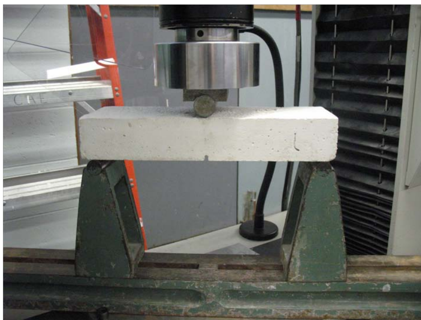
Fig. A.4 - 1– Three point bending set-up for sample cracking
